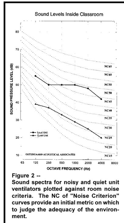
Figure 2 -- Sound spectra for noisy and quiet unit ventilators plotted against room noise criteria. The NC of "Noise Criterion" curves provide an initial metric on which to judge the adequacy of the environment.
